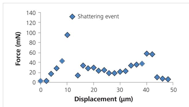
Figure 3: Force displacement plot for the uniaxial compression of a single crystal of HMX shown in Figure 2. The fourth image corresponds to the peak force at 140 mN.
