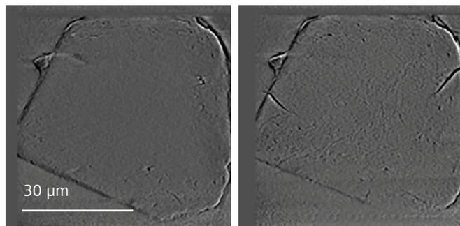
Figure 4: Reconstructed slices through a single crystal of HMX uncompressed (left) and after it has been compressed 5  $\mu\text{m}$  (right). Stress cracks and dislocations are visible in the compressed crystal.
