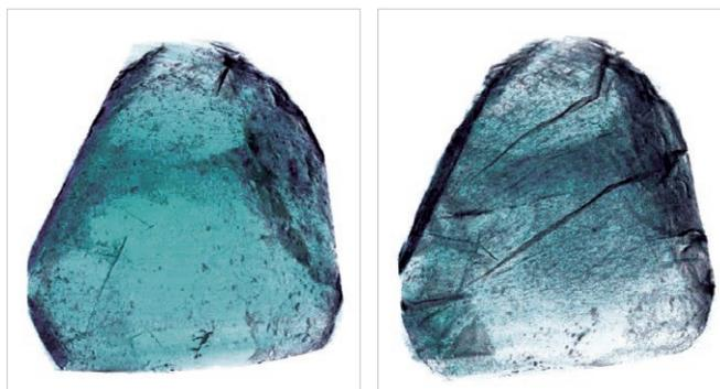
Figure 5: Volume renderings of the same crystal shown above (and on cover) in uncompressed state (left), and after compression (right) by 5  $\mu\text{m}$ . Stress cracks are visible in the compressed crystal.
