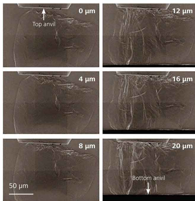
Figure 2: Sequential radiographs as a single crystal of HMX is compressed., shown in 4  $\mu\text{m}$  increments. The top anvil is stationary, while the bottom anvil with the sample mounted on it is moved upwards.
