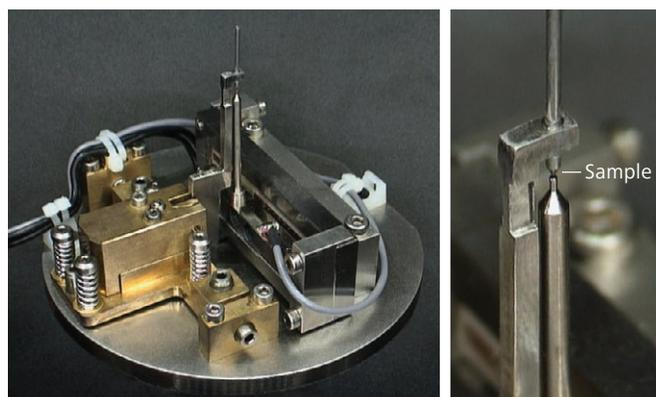
Figure 1: Photo of the load stage (left) and a close up of the top and bottom anvils in uniaxial compression configuration.
