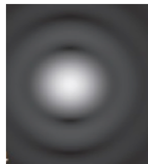
Figure 1b – Spatial Resolution as a Function of Feature Separation. As the same pair of features becomes separated by spacing smaller than the resolution of a system, it becomes indistinguishable as a pair by the imaging system.
