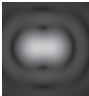
Figure 1b – Spatial Resolution as a Function of Feature Separation. As the same pair of features becomes separated by spacing smaller than the resolution of a system, it becomes indistinguishable as a pair by the imaging system.
